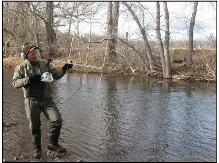
ODFW employee, Kyle Bratcher, pinpoints the exact location of an overwintering radio-tagged early migrant Chinook salmon using triangulation techniques.
